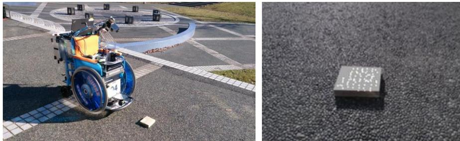
**Fig.7.** The results of detection of 30 [mm] difference in level by the Kinect V2.
