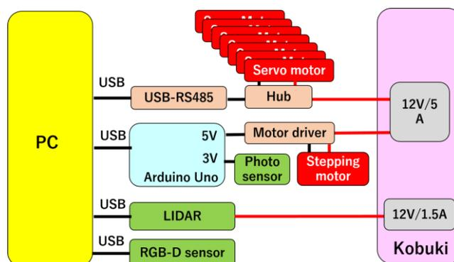
**Fig.4.** The electrical system diagram of Happy Mini
