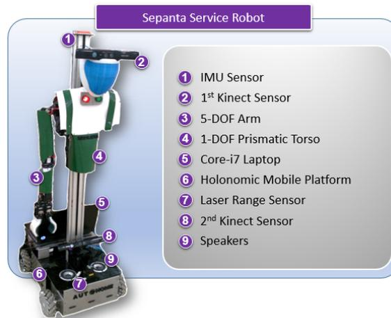
**Fig. 1.** Sepanta II equipment's description.
