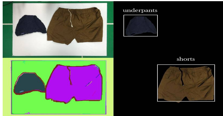
Fig. 3. (Top-Left) An Input Image, (Bottom-Left) Plane Localization and Efficient Graph-Based Image Segmentation, (Right) Output Results
