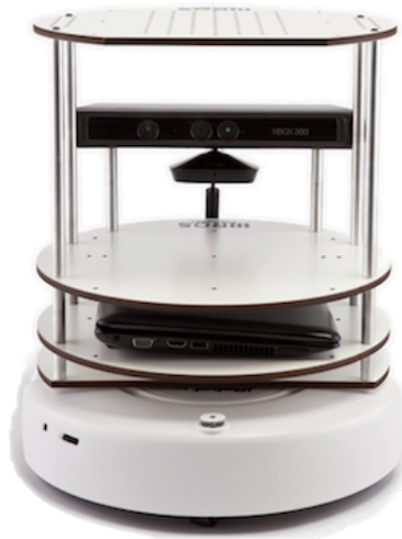
Fig. 1. Conventional TurtleBot mounted on Roomba 4400
