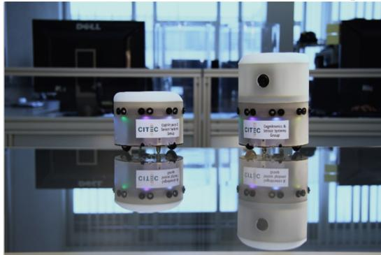
**Fig. 4.** Autonomous Mini Robot (AMiRo) in two different version. Left: Basic Robot. Right: Mounted Kamera Tower
