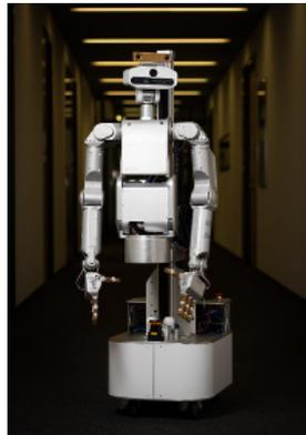
**Fig. 2.** The meka robot platform
