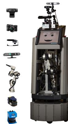
**Fig. 1.** ToBI with its components: camera, 3D sensors, microphone, KATANA arm and laser scanner.
