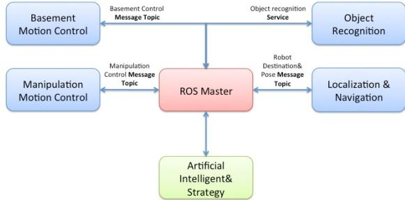
**Fig. 3.** Software framework based on ROS.
