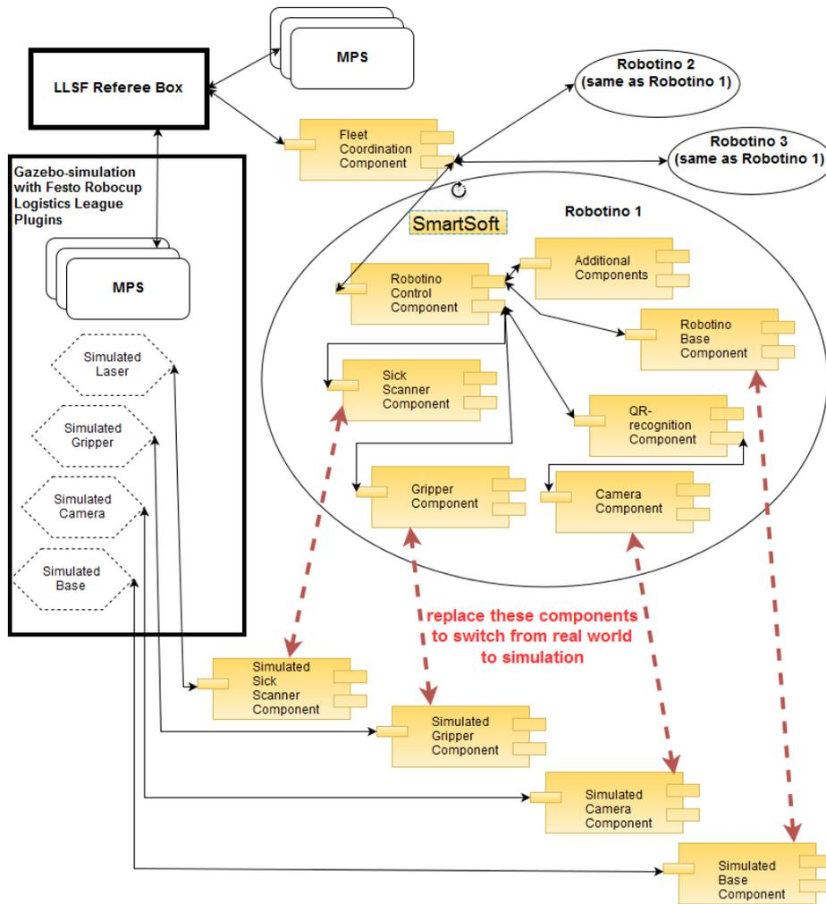
Fig. 3. SmartBots@Ulm component approach for Robocup Logistics League
