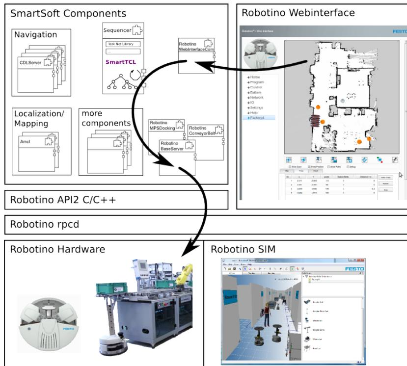
Fig. 2. The Robotino-SmartSoft integration.
