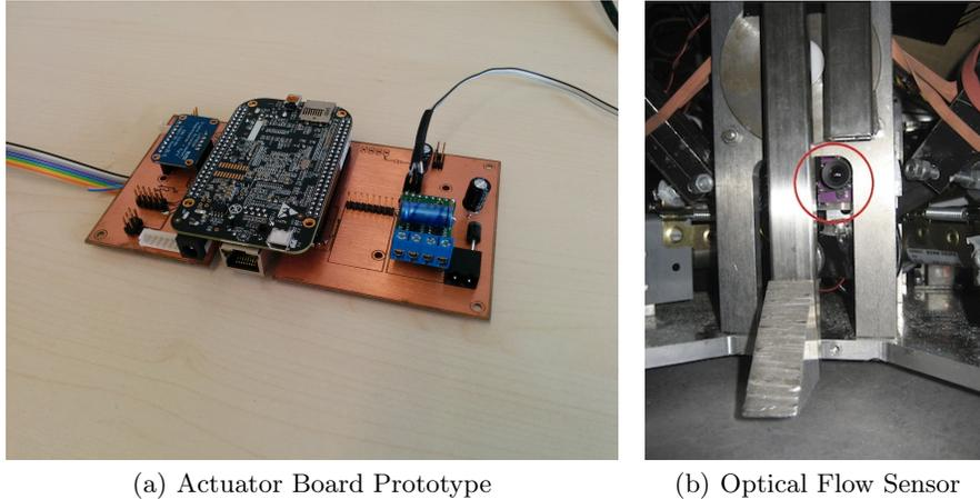
**Fig. 5.** Actuator Board and Optical Flow Sensor
