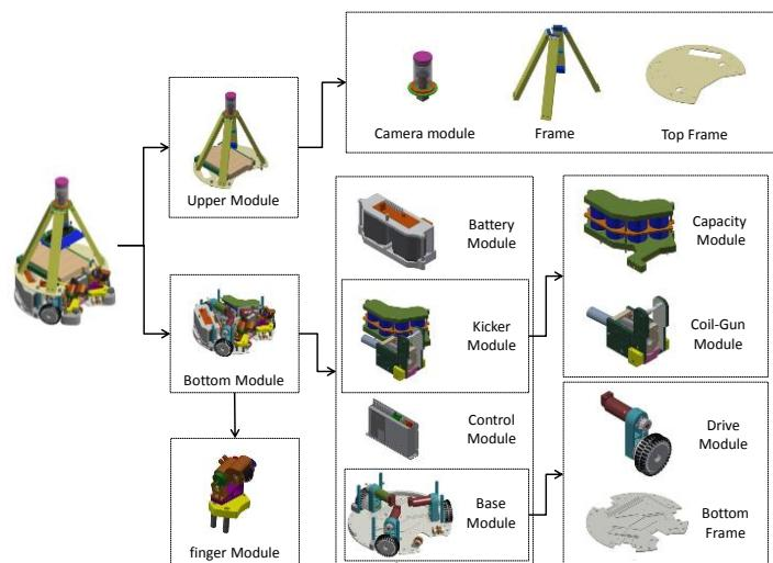
**Figure 1.** “Musashi” robot hardware configuration and modular architecture
