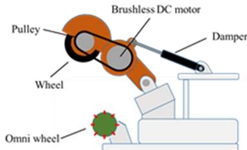
**Figure 4.** Side view of Ball Handling Mechanism
