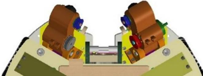
**Figure 5.** Top view of Ball Handling Mechanism
