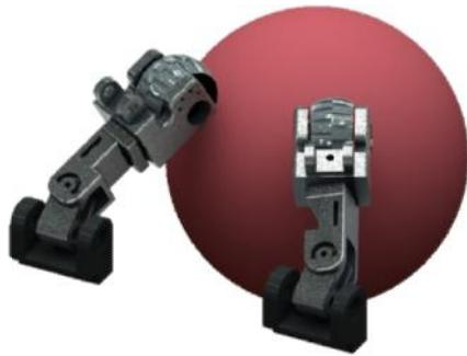
**Fig. 4.** The new ball handling mechanism
