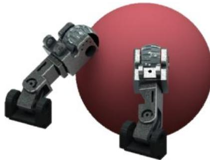
**Fig. 4.** The new ball handling mechanism
