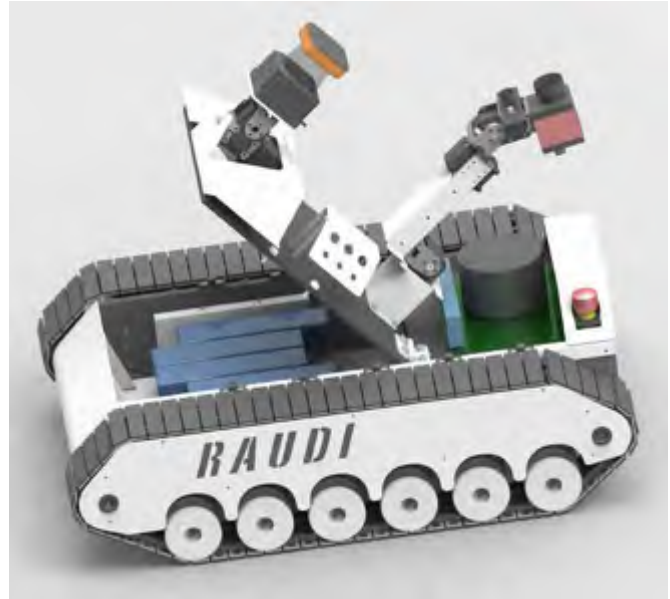
Fig. 10: Rendering of R.A.U.D.I.s CAD model with opened battery cover and removed sheet metal covers.
