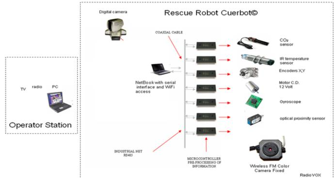
**Fig 6.4** Full system integration of robot's controller, we depicted all sensors & actuators enveloped to complete functionally.
