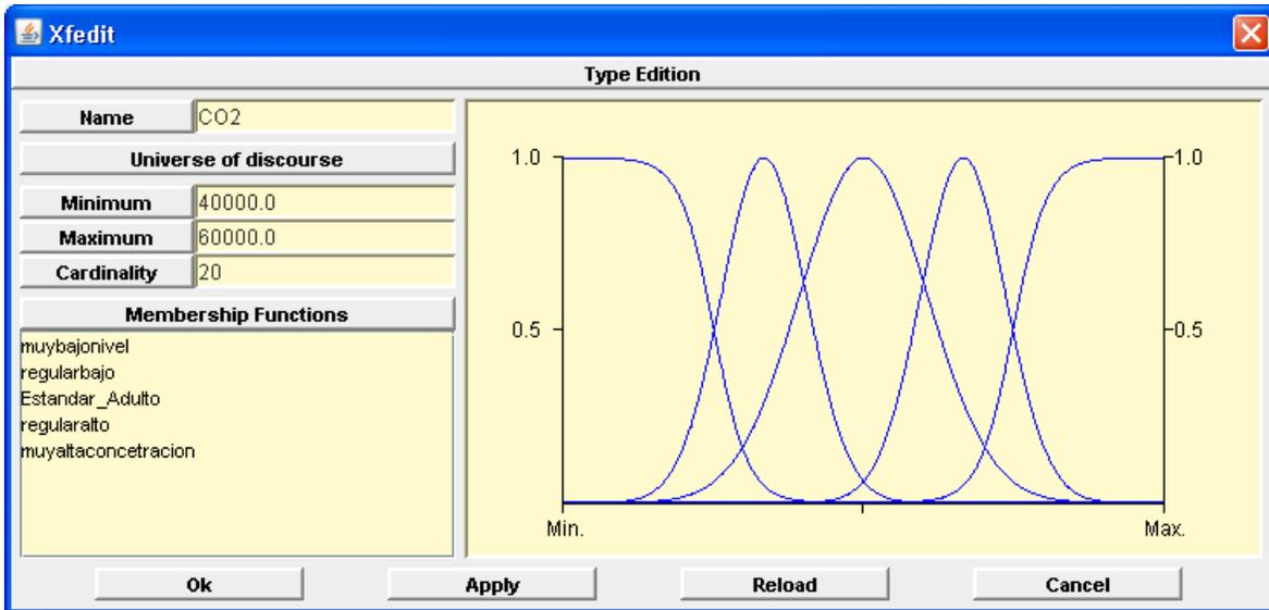
Fig 3.4 Fuzzy graphs typical used for fuzzy controller, Gaussian form are considered in all variables.
