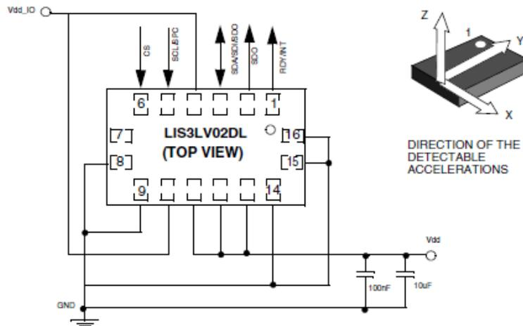
fig 5.2: iSensor based in MEMS 3D level and acceleration [14].
