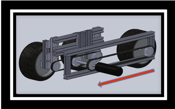
**Fig. 7.3** Robot pulley system used to move one side of symmetrical movement of all wheels by central wheel moved by electrical motor and measured by encoder.
