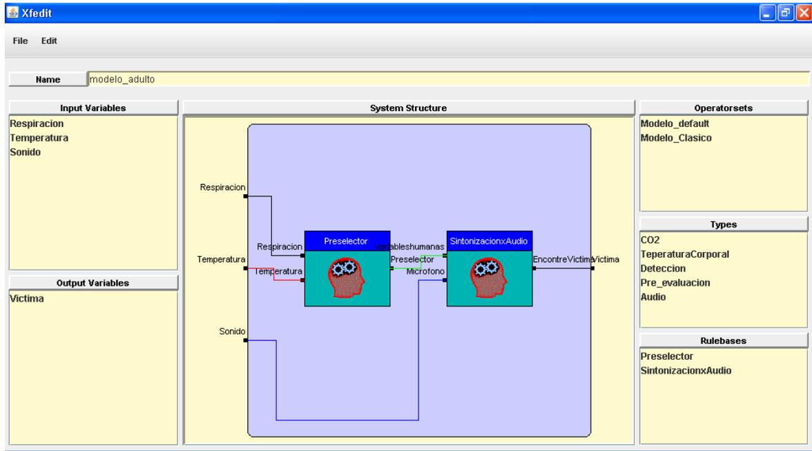
**Fig 3.2** Structure of I/O of fuzzy controller, for this case Pre-selector controller evaluate human variables available CO<sub>2</sub> and temperature; fitting controller evaluate audio voice, this step is changing with old age. This first evaluation steps was developed in fuzzy type I style, as reference as start point to variable evaluations [22].
