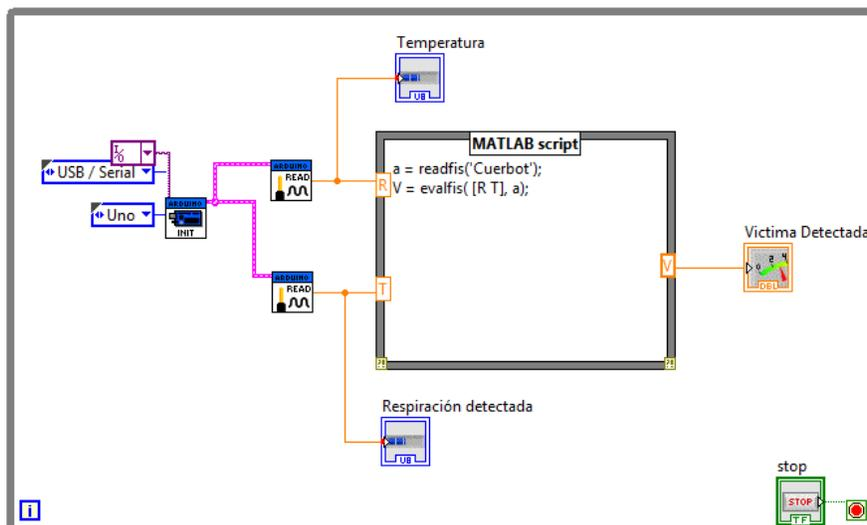
Fig 3.7 Fuzzy System Type I with hardware interface with Arduino microcontroller, integrating control and victim indicator.
