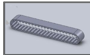
**Fig 7.6** Toothed band gear and pulley used in this project.
