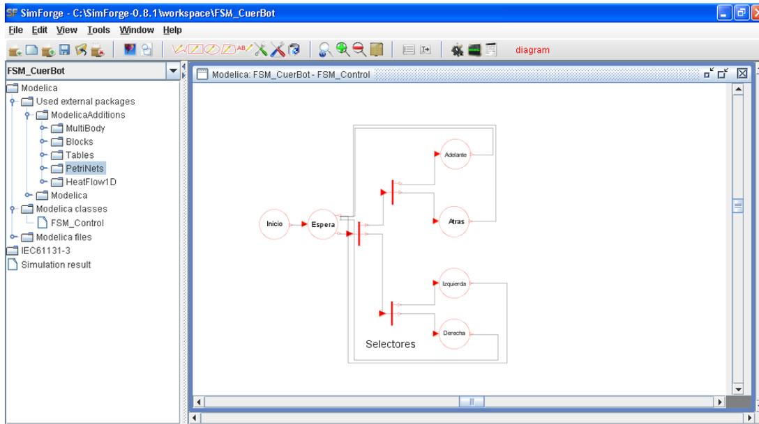
**Fig 3.8** FSM algorithm tested by SimForge tool for manual control of robot displacement, this figure depicts Petri Net equivalent for general structure [23,24].
