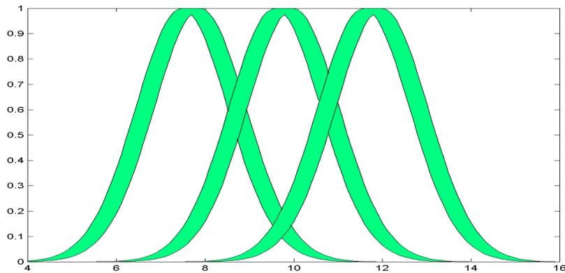
**Fig 3.1** Temperature type-2 membership functions, it's a simple example of temperature evaluation.
