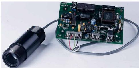
**Fig.6.1** IR Sensor model OS65 used for body temperature measurement
