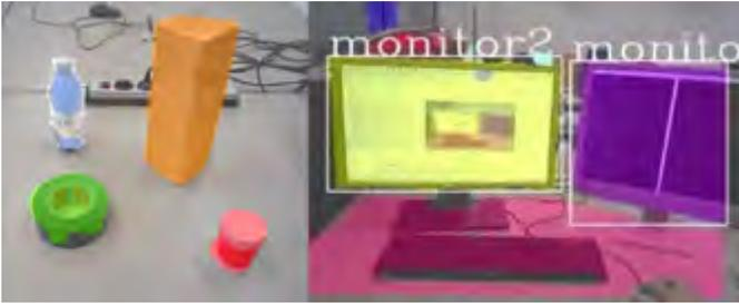
Fig. 12: Real-time segmentation for clustering a depth image (left) and object detection based on partial views (right).
