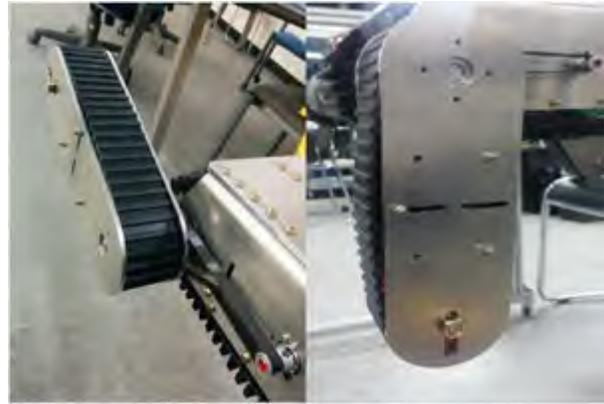
Fig. 4. Photo of robot's sub-rubber track
