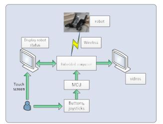
Fig. 16 Hardware structure of control box
