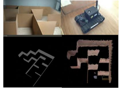
In the same time we are developing method of generating 3D map by Kinect 360 device assembled on out two-wheel robot. Fig 11 shows the 3D map example.
