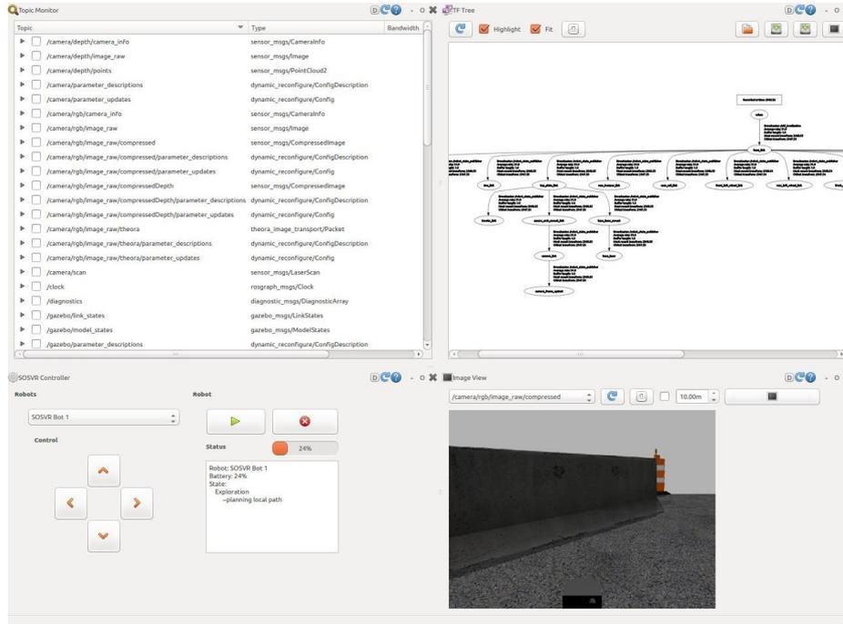
Figure 2. Dashboard-rqt robot state visualizer and controller
