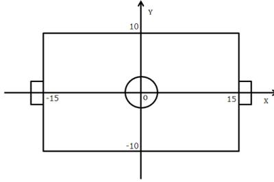
**Fig. 2.** An orthogonal coordinate system is defined in the field in order to determine the position of foe-agents in the place close from our team's goal. The new orthogonal system has the center of the center circle as the origin and has negative value of  $x$  coordinate for our area in the soccer field and is  $x = -15$  at our goal mouth, where our area is taken as the left side in the field.
