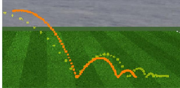
**Fig. 3.** The result of the prediction on the movement of the ball. The orange dots and the light green dots represent trajectories of the ball by our estimation and of the real carrying the ball, respectively.
