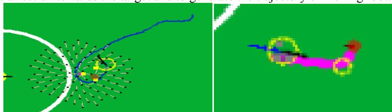
Figure 9: Motion: Potential Field (left); Footstep planning (right)
