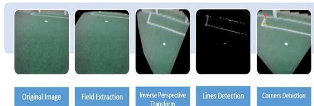
Figure 5: Detection of field, lines and corners
