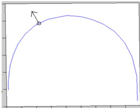
Figure 2: Approximated Foot contour with Bezier curve
