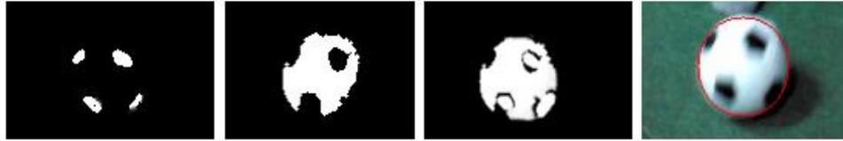
Figure 7: Color Based Ball Detection
