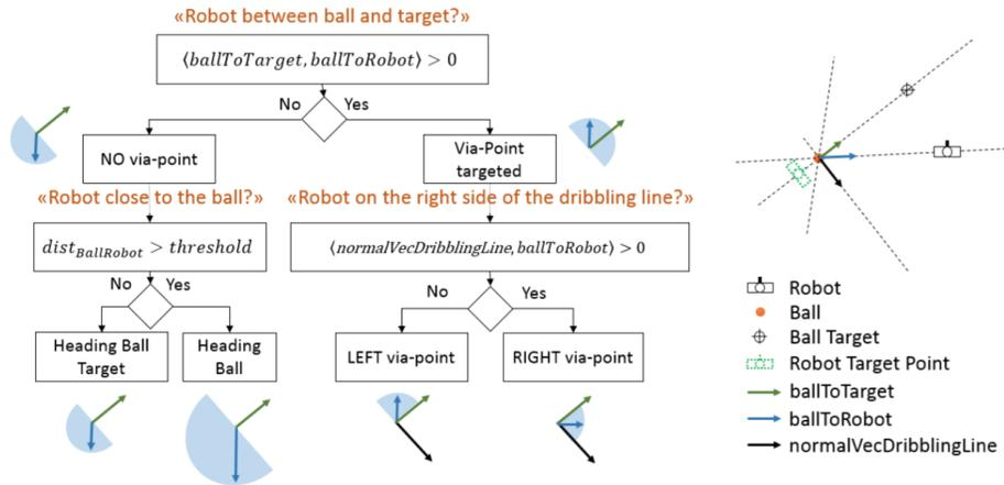
**Fig. 3.** Decision tree of walkToBall, part of the Z-Knipsers’ dribbling skill. This tree determines based on the locations of robot, ball and target, how the robot approaches the ball.
