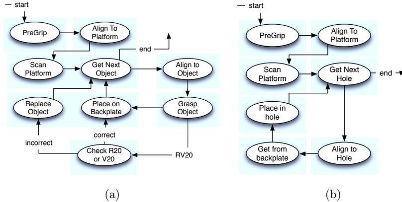
Fig. 5: (a) The simplified subtask-state-machine that is used for grasping objects at a service area. (b) The simplified subtask-state-machine that is used for dropping objects into the holes for PPT.
