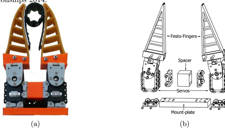
Fig. 2: Figure (a) illustrates the adaptation of the gripper to the round shape of the object. Figure (b) shows a drawing of the separate parts of the new designed gripper in more detail.
